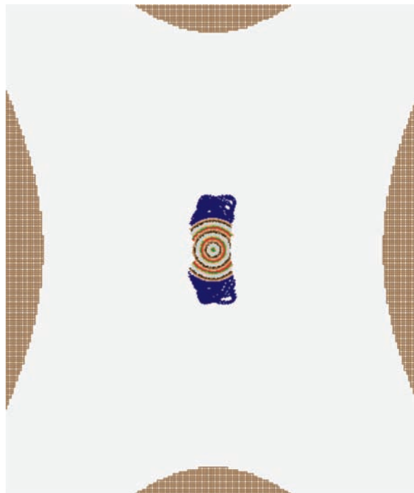
Figure 3. Close up of center of SIMION electrode array used to simulate ion trajectories. The time an ion spends in each of 30 cylinders in the center of the trap was recorded to produce a distribution of probability as a function of radius. An ion trajectory at q_z = 0.10 is shown, where the ion color is changed in each of the 30 cylinders for emphasis. The blue trace on the top and bottom of the cylinders is the ion path outside of the cylinders. The left and right electrodes are the end-caps through which ions enter and exit the trap. The top and bottom electrodes are actually one cylindrical ring electrode where the trapping voltage is applied.
